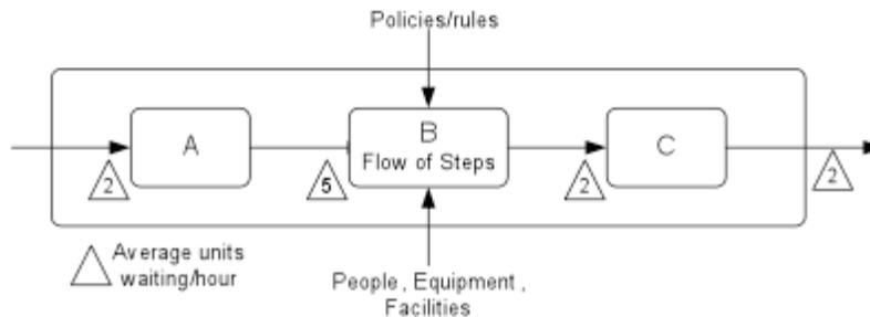
Figure 1. A simple process with a constraint or bottleneck
