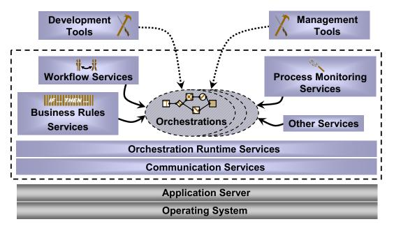
As the diagram shows, BPM server vendors commonly build their offerings on an application server, such as the .NET Framework or a J2EE-based product, which in turn runs on some operating system. On this foundation, a BPM server can provide a range of support for orchestrations, including the following:
